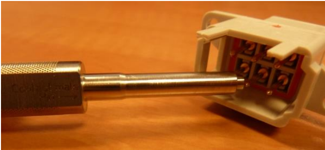
Pin contact extraction process
