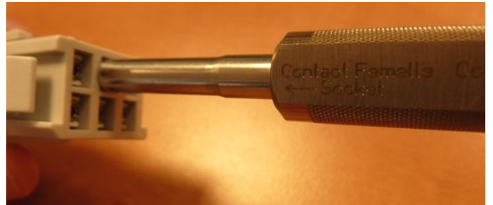
Socket contact extraction process
